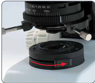
Close the Koehler field diaphragm
