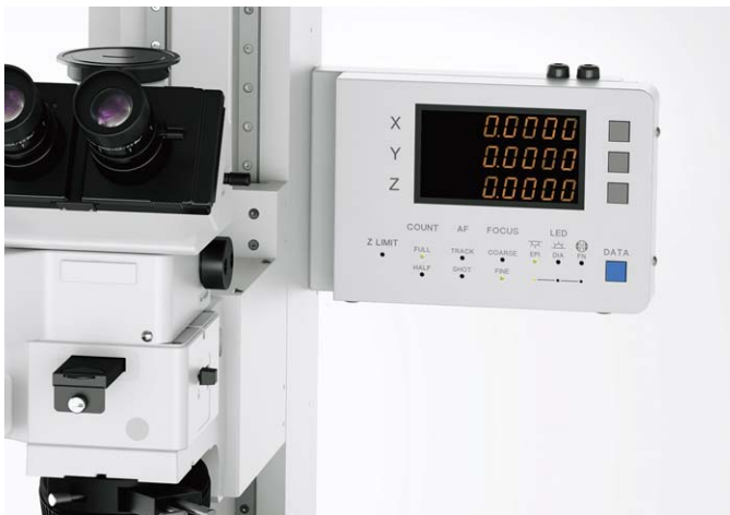
Digital readout attached to the frame
