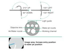
This zoom gastroscope features the well-known 135 x Multi Zoom which leads to clear and more detailed visualisation, allowing deeper analysis of mucosal structures. It has a small bending radius and similar functionality to the routine gastroscope including all features.
